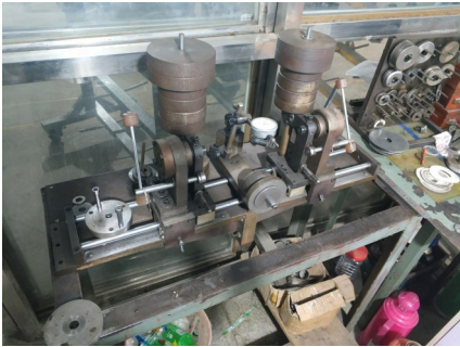
图3 圆锯片横向刚度测试装置 Fig.3 Testing device for transverse stiffness of circular saw blade
